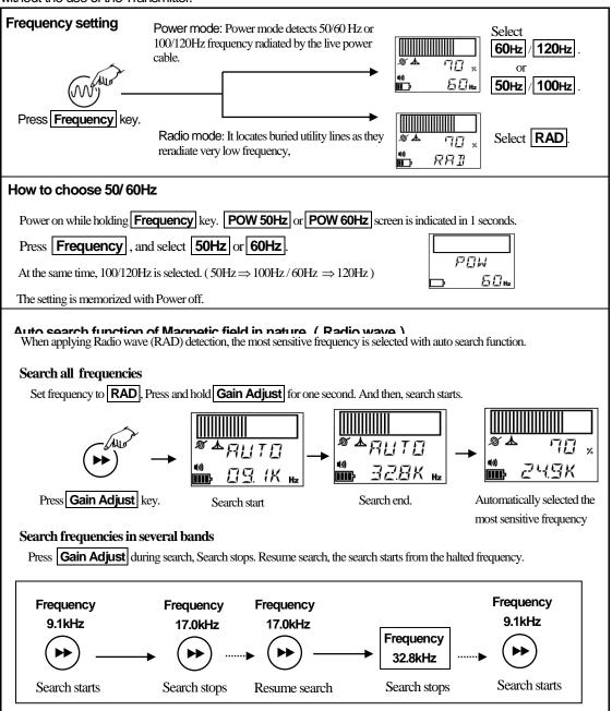
Above mentioned example shows the first search detects the most sensitive frequency from 9.1k to 17kHz. And then search is halted. Then, search resumes. The second search detects the most sensitivity frequency from 17k to 32.8kHz Applying this function, several different kinds of cables can be detected in several stages.
