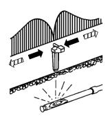
**Depth measurement**  $\Rightarrow$  Press **DEPTH** key
