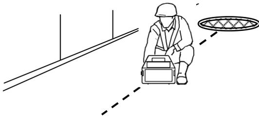
Do not place the Transmitter on a manhole cover or other steel covering.
