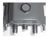
13.Before replacing pump manifold (29), first rotate crankshaft (18) until two outside plungers (24A) extend evenly forward. Lubricate ceramic plungers with a light film of oil. Carefully and evenly slide manifold over plungers and press manifold firmly against crankcase (1). Replace manifold stud bolts (45), washers (47) and nut (46) and tighten to 59 ft.-lbs.
