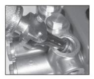
Use a small slide hammer to remove valve seats (37) from manifold (29). Inspect valve plate (36) and valve seats (37) for wear. If excessive pitting is seen, replace the worn parts. Check valve seat o-ring (38) for wear and replace as necessary.
