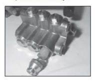
Remove the inlet valve retainer assembly (34A-39)
