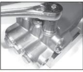
With a 22mm socket, remove the three discharge (43) and three inlet (41) manifold plugs.
