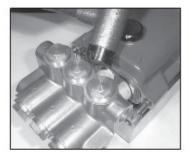
Tap the back of the valve casing (29) with a rubber mallet.
