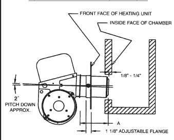
THE AIR TUBE LENGTH (DIM A) IS THE DISTANCE FROM THE FRONT OF AIR TUBE RETAINER FLANGE TO FACE OF AIR CONE. NOTE ADJUSTABLE FLANGE WIDTH.
