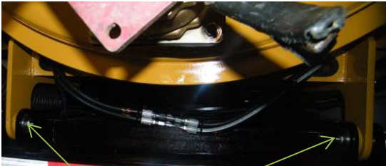
TANK PIVOT TUBE GREASE POINT
