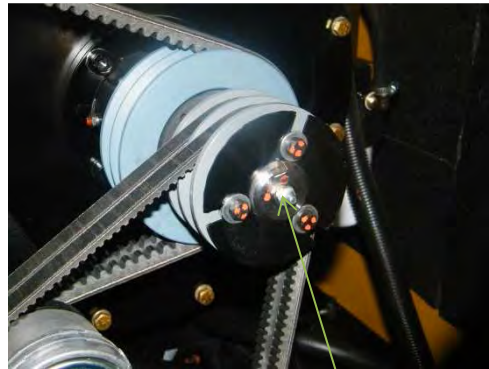
ENGINE GREASE POINT
