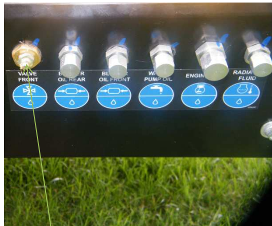
4-WAY VALVE GREASE POINT
