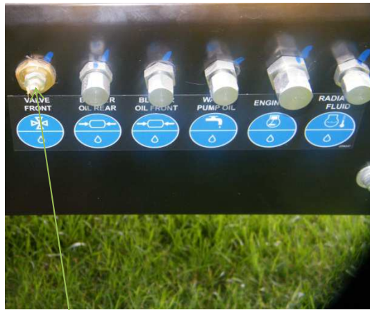
4-WAY VALVE GREASE POINT
