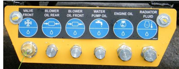
4-WAY VALVE GREASE POINT
