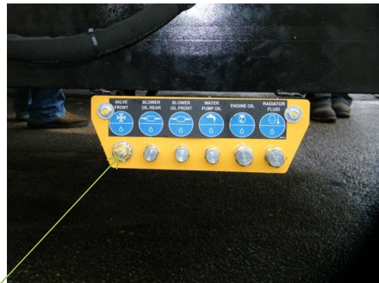
4-WAY VALVE GREASE POINT
