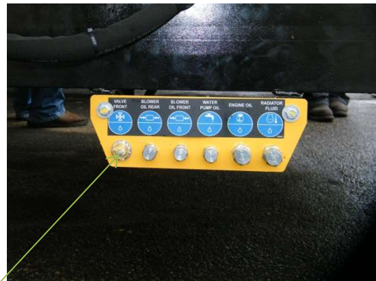
4-WAY VALVE GREASE POINT
