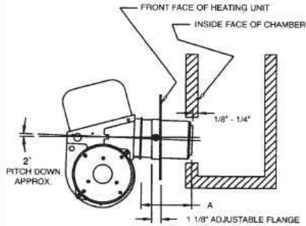
THE AIR TUBE LENGTH (DIM A) IS THE DISTANCE FROM THE FRONT OF AIR TUBE RETAINER FLANGE TO FACE OF AIR CONE. NOTE ADJUSTABLE FLANGE WIDTH.
