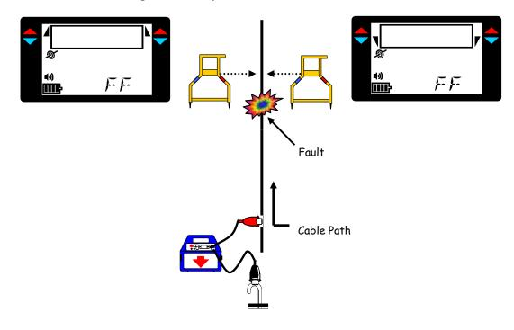
To confirm the fault place the red leg over the suspected faulted area. Pivot the A-frame in a 360-degree circle if the indicator continually shows Red then fault is beneath the red leg.
