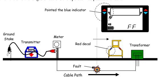
Move backwards placing the A-frame in the earth every few inches when the arrow changes direction again you have reached the area of the fault. The fault point will be in the center of the A-frame.
