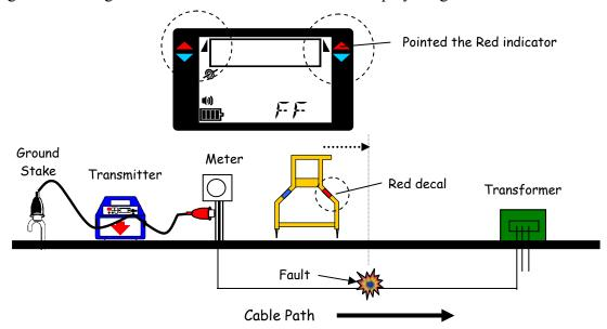
When the arrow changes directions the operator has passed the fault.
