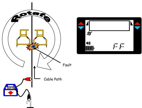
**Multiple Faults** –Place both legs of the A-frame in the ground with the red leg directly over the fault point. With a line that has multiple faults, the fault that registers the highest reading on the display is the fault. That needs to be repaired.
