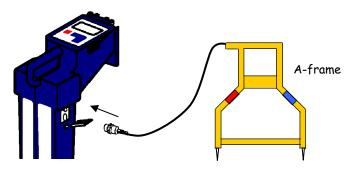
Place both legs of the A-frame in the earth with the red leg pointing at the ground stake. Distance from ground stake should be approximately the same as the suspected depth of the cable.
