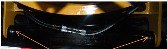
TANK PIVOT TUBE GREASE POINT
