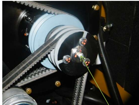
ENGINE GREASE POINT
