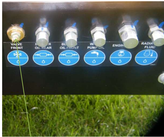
4-WAY VALVE GREASE POINT
