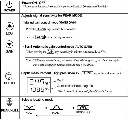
**PEAK & NULL MODE:** Maximum sensitivity is the point directly above the object line and the buried object line location is indicated with arrow.
