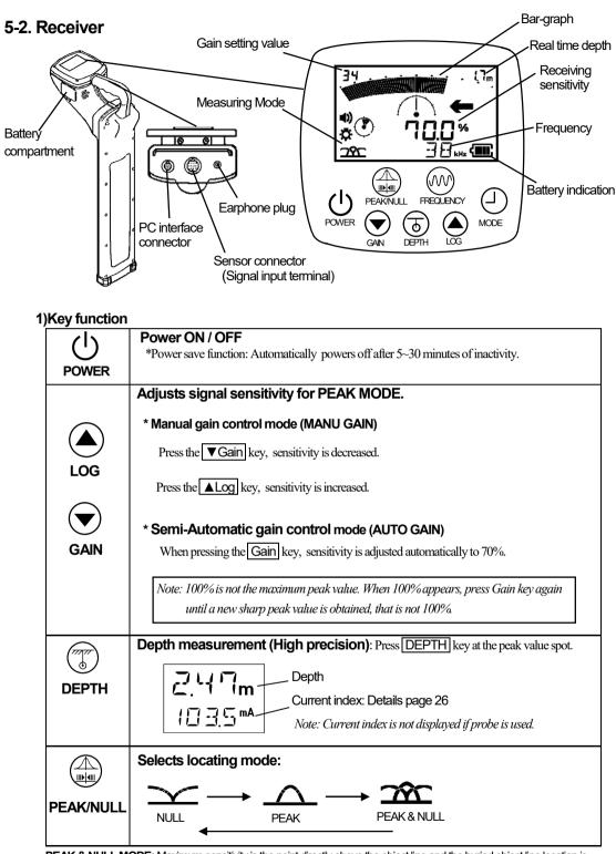
PEAK & NULL MODE: Maximum sensitivity is the point directly above the object line and the buried object line location is indicated with arrow.
