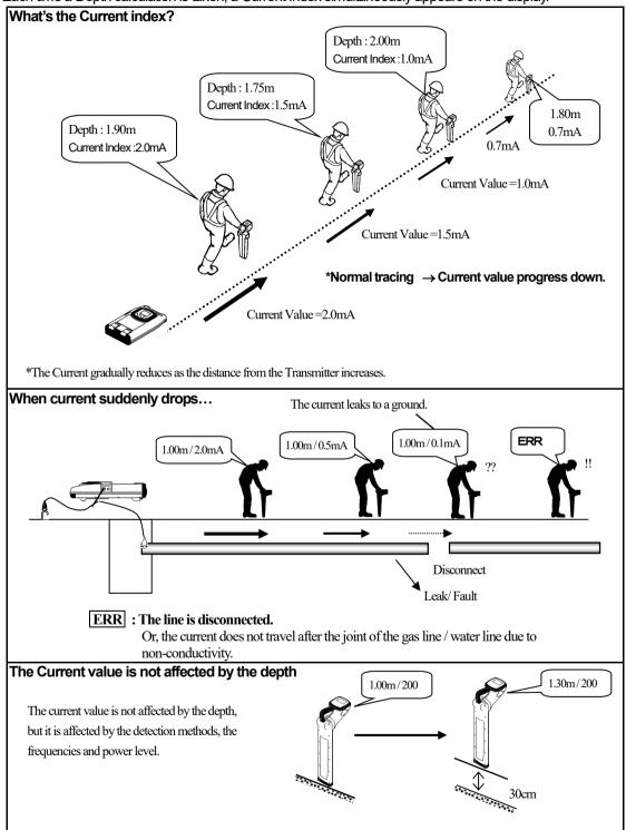
Each time a Depth calculation is taken, a Current Index simultaneously appears on the display.
