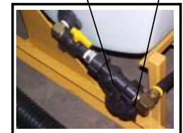
Ball Valve in On Position
