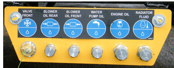
4-WAY VALVE GREASE POINT
