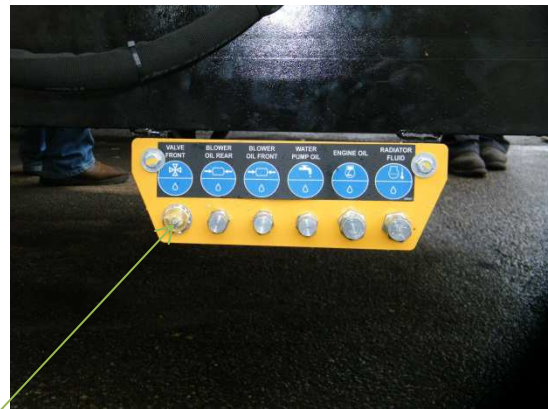
4-WAY VALVE GREASE POINT
