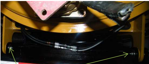
TANK PIVOT TUBE GREASE POINT
