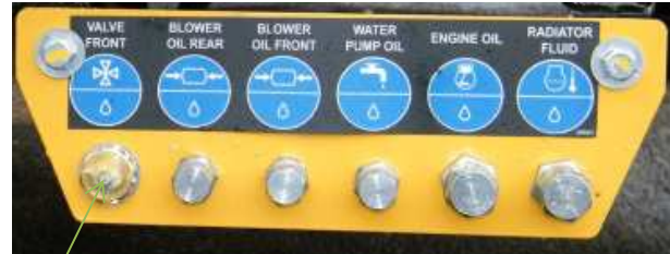
4-WAY VALVE GREASE POINT
