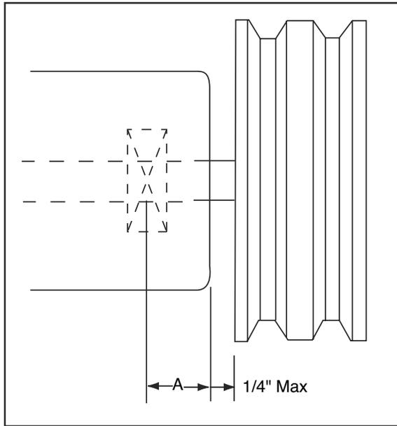
$$\text{Belt Pull lbs} = \frac{252100 \cdot \text{Motor HP}}{\text{Blower RPM} \cdot \text{Sheave Diameter}}$$
