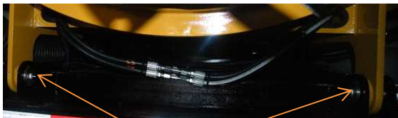
TANK PIVOT TUBE GREASE POINT
