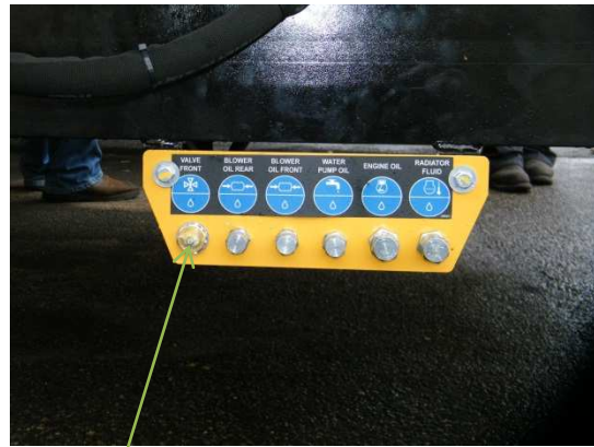
4-WAY VALVE GREASE POINT
