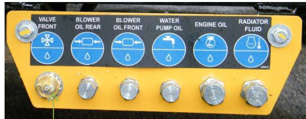
4-WAY VALVE GREASE POINT
