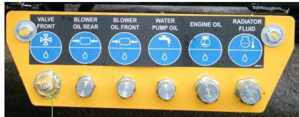
4-WAY VALVE GREASE POINT
