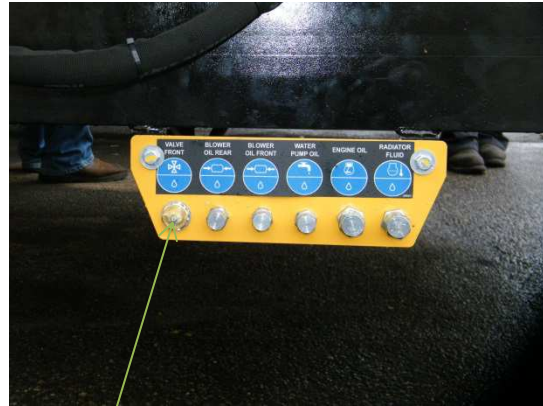
4-WAY VALVE GREASE POINT
