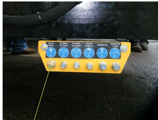
4-WAY VALVE GREASE POINT
