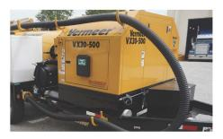
**NO HASSLE HOSE.** Hang the suction hose on the side of the machine when moving between jobsites instead of coiling or disconnecting it, increasing productivity and reducing operator fatigue.
