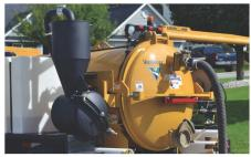
THREE STAGE CYCLONIC FILTRATION. Engineered to prolong filter and blower life, the system is suitable for wet and dry applications. The cyclones use a tuned vortex system in which the outer vortex spiral forces small particles to fall into a separate canister. The filtered stream then passes up through the inner cyclone tube and carried to the final poly filter.
