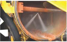
**IN-TANK WASH-DOWN.** Delivers a highpressure water spray to the tank interior helping simultaneously dump material and clean the inside of the tank. Saves clean up time and makes it easier to remove difficult debris.
